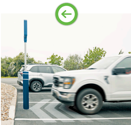
Vehicle impacts BumperSign FlexPost.
