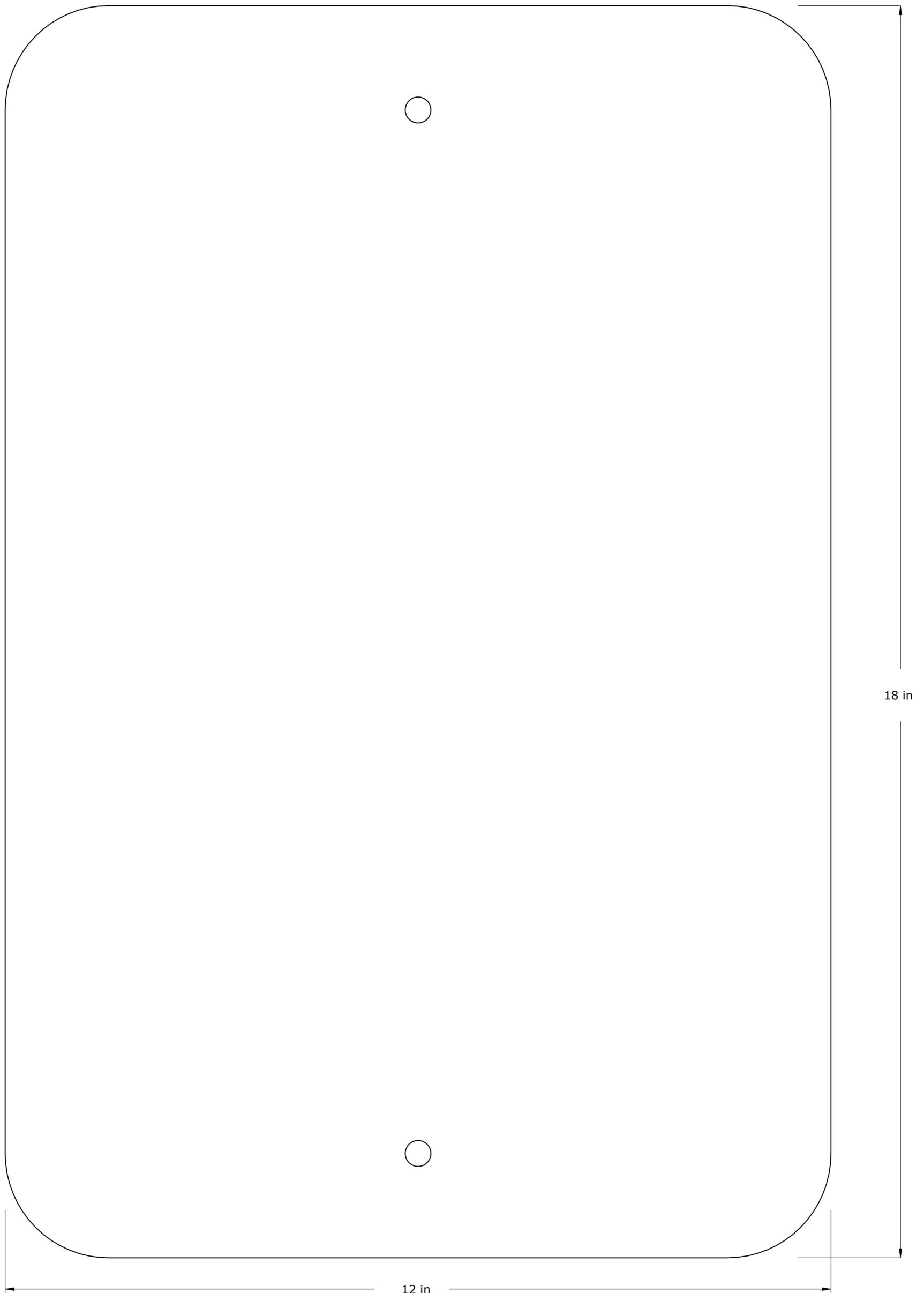
HOLES: TWO  $\varnothing 0.375$ " HOLES ARE CENTERED, LOCATED 1.5" FROM TOP AND BOTTOM EDGE.
